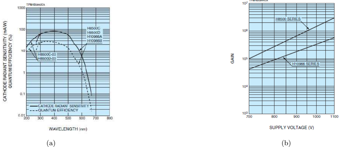
Figure 3.17: (a) Typical spectral response for the MAPMT (H8500D) used and (b) typical gain [68].
