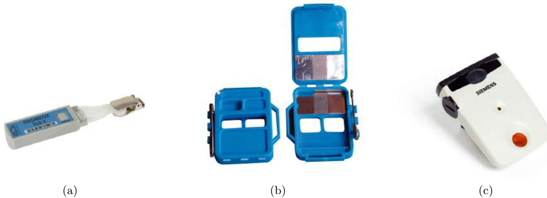
Figure 1.3: Examples of dosimeters: (a) TLD [18], (b) Film Badge Dosimeter [19] and (c) EPD [20].
