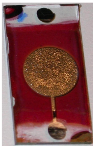
Figure 6.11: A P3HT:PCBM cell after the deposition of Al electrode and the annealing carried in glove box.
