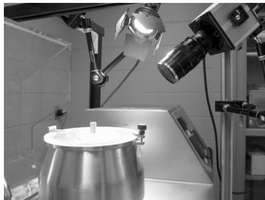
Fig.4.1. Picture of the experimental apparatus for the measurement of the powder surface velocity
