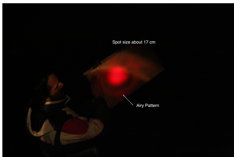
Figure 3.5: Spot size on the 13km link.
