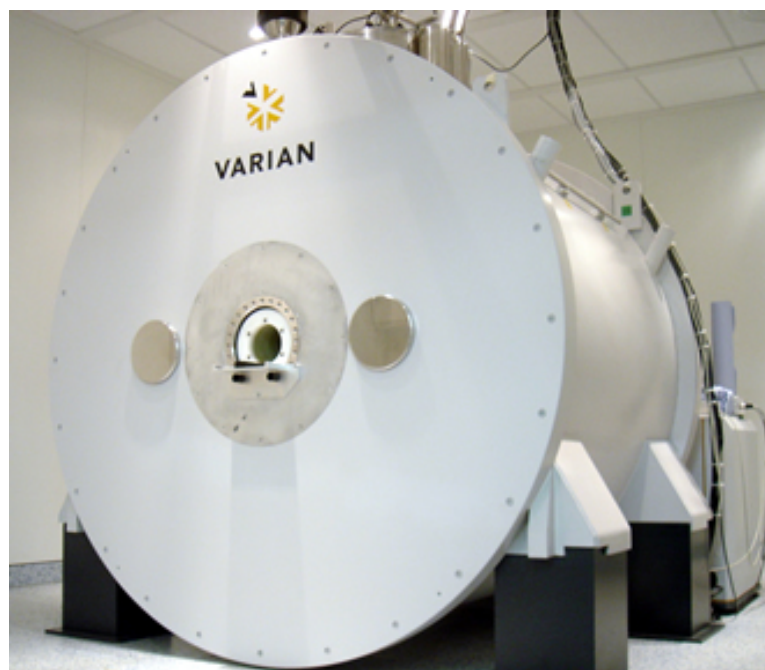
Figure 14. Experimental MRI scanner (Varian 9.4T) employed in the study. It utilises a much higher magnetic field compared to a typical clinical scanner and acquires images with less than 40 micron resolution.
