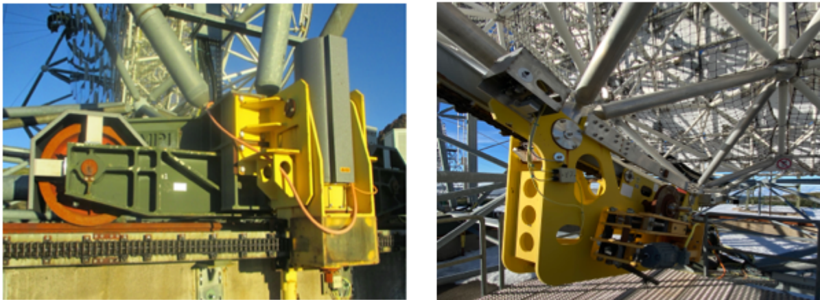
Figure 2.11 Left: one of the six mechanical bogies that allow the azimuth rotation of the telescopes. Right: the elevation drive, located at the center of the structure and behind the reflective surface.
