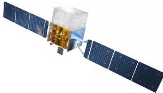
Figure 1.12 An artistic impression of the Fermi satellite with its Large Area Telescope (LAT) shown on the top. Image credit: NASA.
