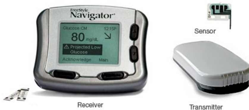
Figure 1.3: FreeStyle Navigator CGM System[45]. Miniature electrochemical sensor placed in the subcutaneous adipose tissue (bottom left), a disposable sensor delivery unit (top right), a radiofrequency transmitter connected to the sensor (bottom right), and a hand-held receiver to display continuous glucose values.
