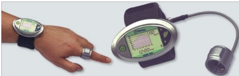
Figure 2.3: OrSense NBM-200G [82]. On the right are visible the annular probe linked to the computation unit.
