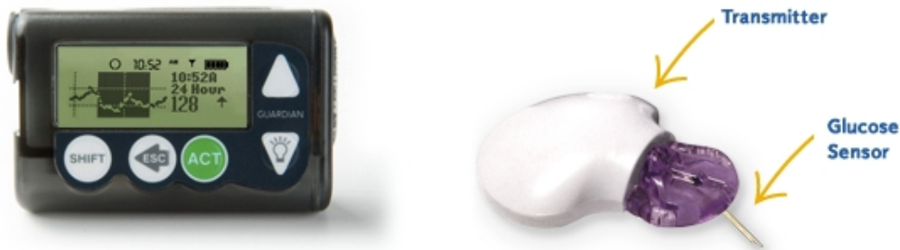
Figure 1.5: The Guardian REAL-Time [50]. REAL-Time CGM System monitor (left), the MiniLink REAL-Time Transmitter together with the glucose sensor inserted in the subcutis (right).
