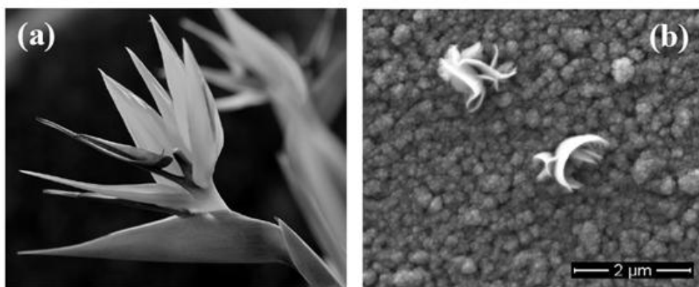
Figure 4. The Strelitzia flower (a) and SEM micrograph of \alpha -SWCNH/TiO 2 (PVD) (b) showing the first examples of strelitzia -like titania via PVD.
