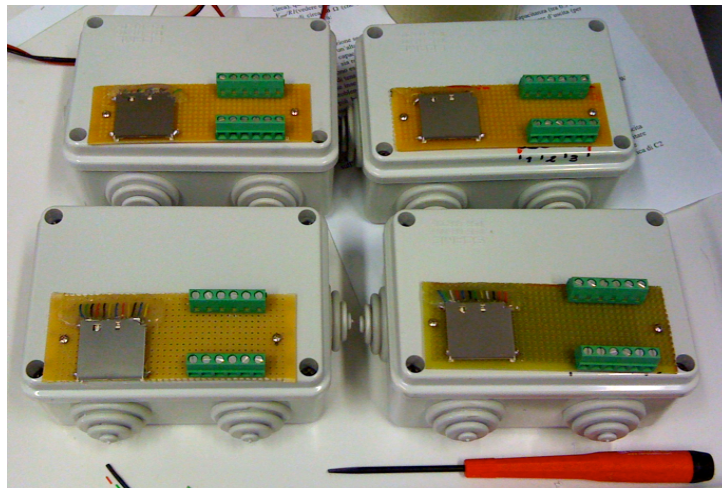
Fig. 3.7 Picture of the dataloggers. The input and output contacts of the probes, and the SD Card Slot are outside the box for convenience.
