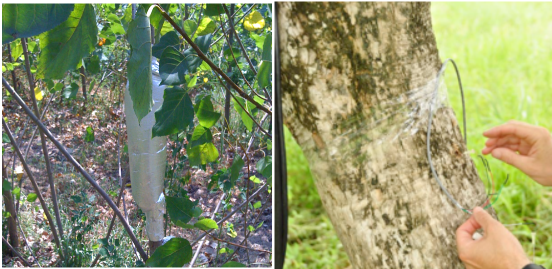
Fig. 3.4 Installation of Granier probes in two different sites. Left image: Pontedera, Pisa - Italy: It is visible the TermoFlex used to prevent the heating of the trunk due to solar radiation. Right image: CATIE - FUNCiTREE project, Costa Rica: probes are being inserted into a tree trunk.
