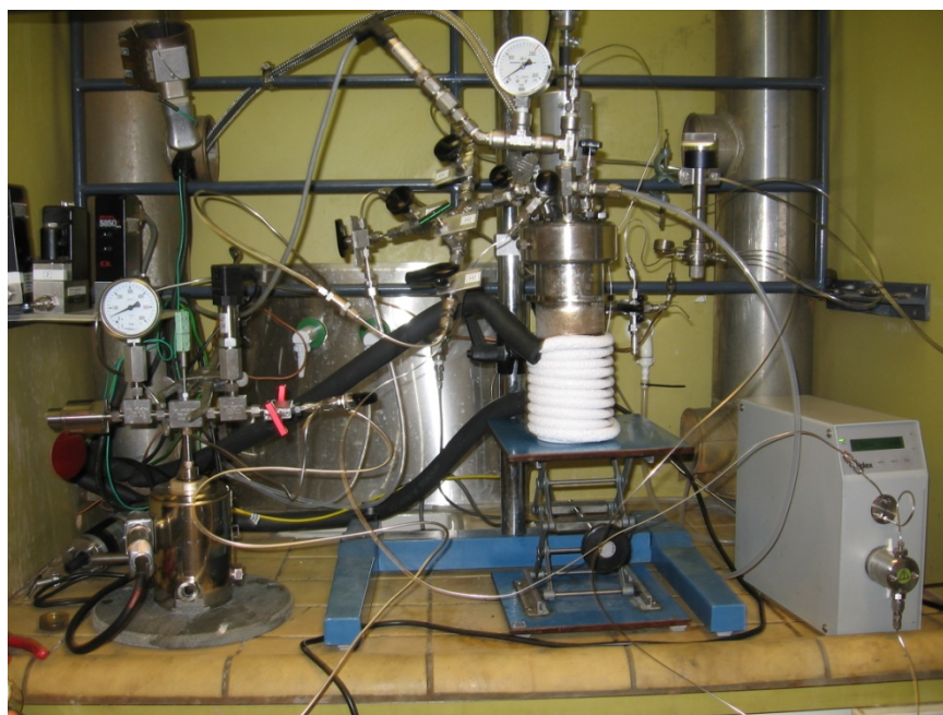
Figure 2.17. Representation of the batch reactor set-up for kinetics studies.
