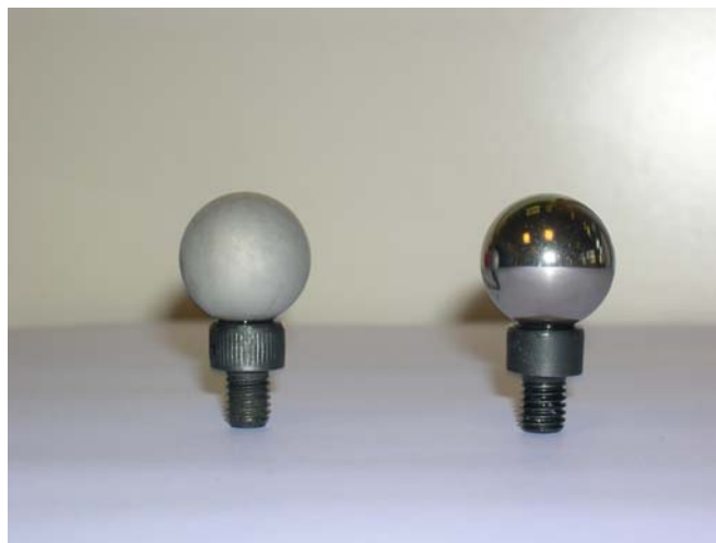
Fig. 4.10: Stainless steel balls with (left) and without (right) acid treatment.
