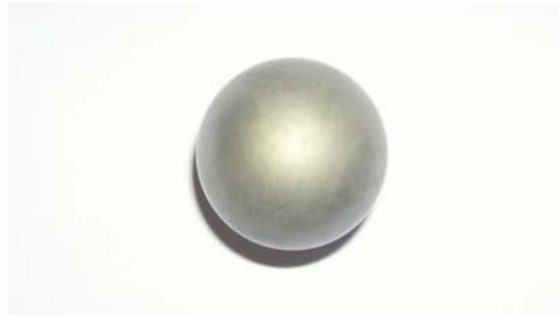
Fig. 4.11: Acid-etched stainless steel after 4 days.
