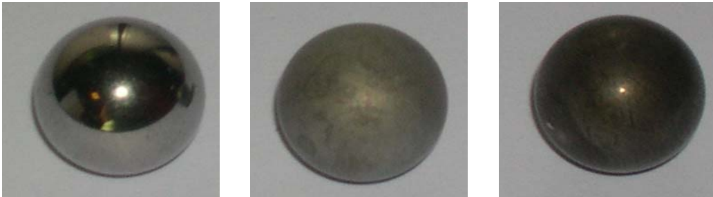
Fig. 4.9: From left to right: steel sphere without treatment, immediately after the acid-etching and after some hours.
