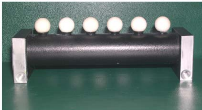
Figure 4.20: Ball bar with spheres made of alumina
