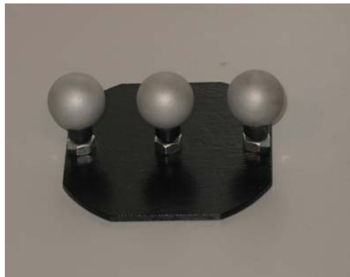
Fig 4.22: Prototype of ball bar artefact for ISO10360-2.
