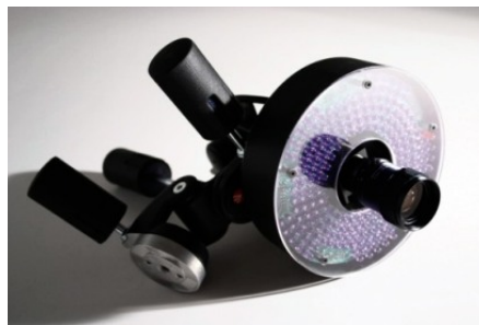
Figure 2.5: Camera with infrared illuminators.
