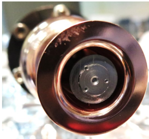
Figure 7.5 Bottom view of the “compact magnetron sputtering source”. Centering the cathode with respect to the cavity is very important in order to have a symmetrical deposition process.
