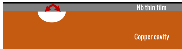
Figure 3.4 The heat flow in thin film will be transmitted only unidimensionally and cannot by-pass the thermal defect.
