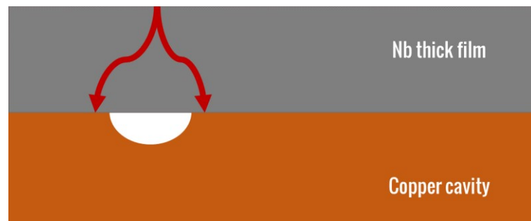
Figure 3.5 The heat flow in thick film could be transmitted more tridimensionally and can easily shunt the defect at the interface
