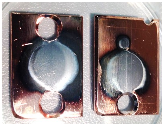
Figure 7.17 Two of the samples used for the BCP test. The etching rate on the sputtered films is 1,4 \mu\text{m}/\text{min}
