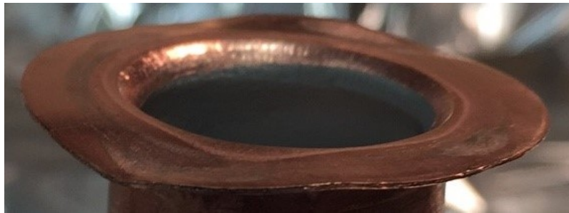
Figure 7.10 Flange deformation due to high temperature (650 °C). The copper becomes softer and lose his mechanical properties. A deformed flange is a very probable source of vacuum leaks, avoiding the possibility of the rf test.
