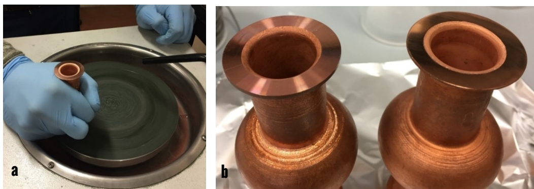
Figure 4.2 Lapping of the flanges (a). The flange surface appearance after the lapping process (b).
