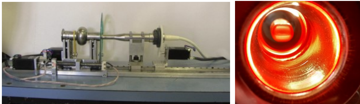
Figure 6.4 Picture of the optical inspection system on the left. Picture of the camera, inside the cavity, during an optical inspection on the right.
