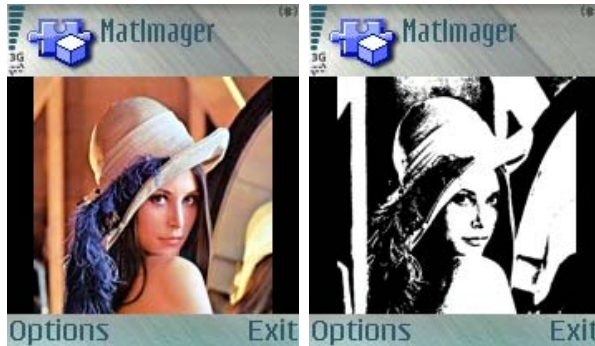
Figures 7a and 7b: Matlmager on a Nokia N70 Smartphone for image thresholding
