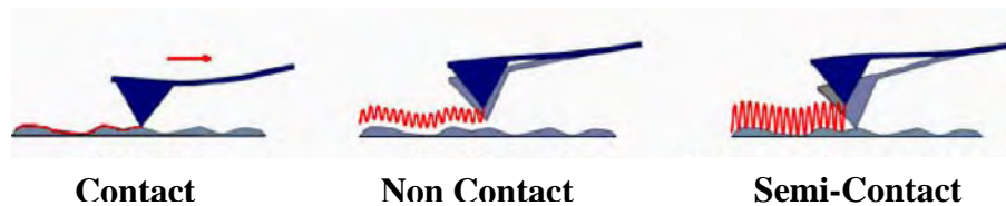
Figure 41: Scheme of the AFM working modalities. In contact mode the topography is obtained by the cantilever bending; in non contact mode and semi-contact (or tapping) mode the signal comes from the variation of frequency, magnitude and phase of the cantilever oscillation.
