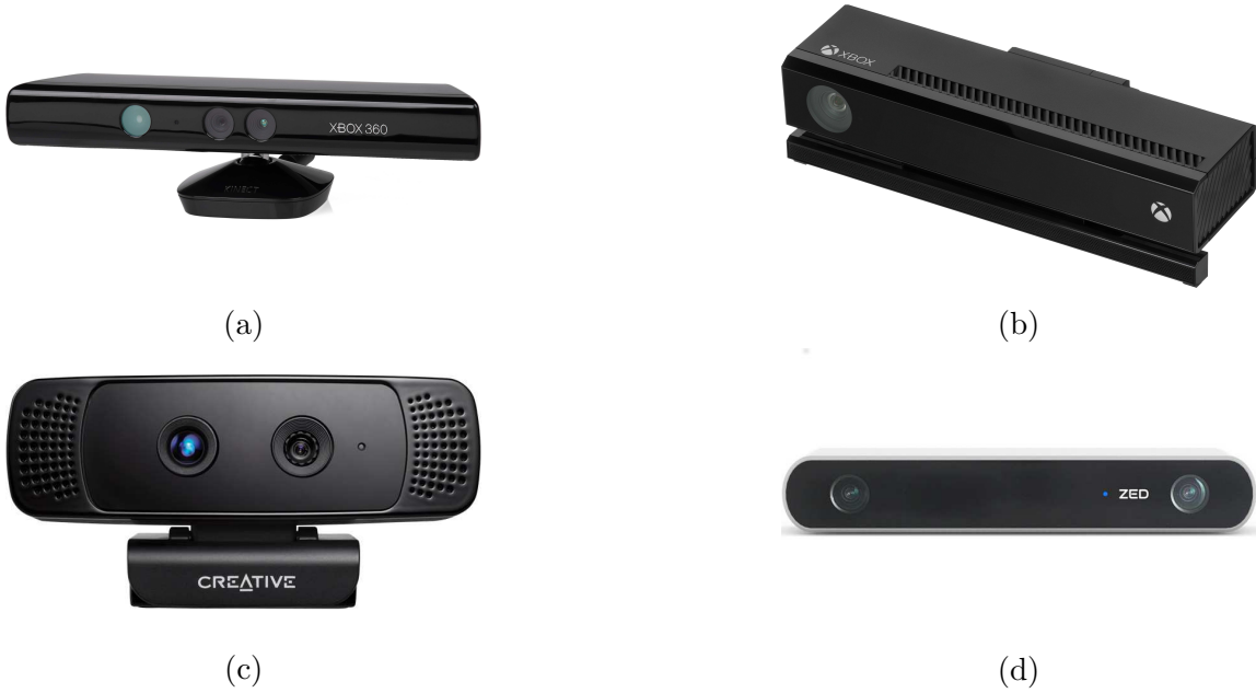
Figure 2.2: Examples of consumer depth cameras: Microsoft Kinect v1 (a), Microsoft Kinect v2 (b), Creative Sens3D (c), StereoLabs ZED (d).
