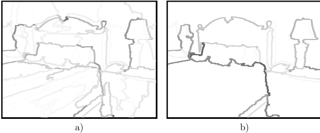
Figure 4.4: Similarity values b_{i,j} computed on a sample scene: a) b_{i,j} values between segments in the initial over-segmentation; b) b_{i,j} values between segments at the end of the merging procedure. The color of the boundary between any two touching segments is proportional to their similarity score (white corresponds to high b_{i,j} values and black to low ones).
