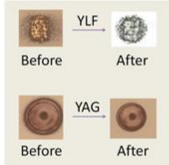
Figure 20. Burn paper images of both laser beams directly before and after passing through the beam combiner.
