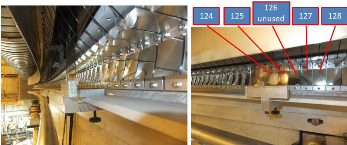
Figure 27. Polarizers installed on fibres 124 and 125 of JET HRTS optical fibre array.
