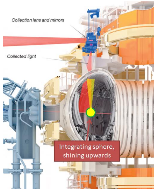
Figure 35. Depiction of post-experiment full emission calibration using a large integrating sphere tungsten light source.
