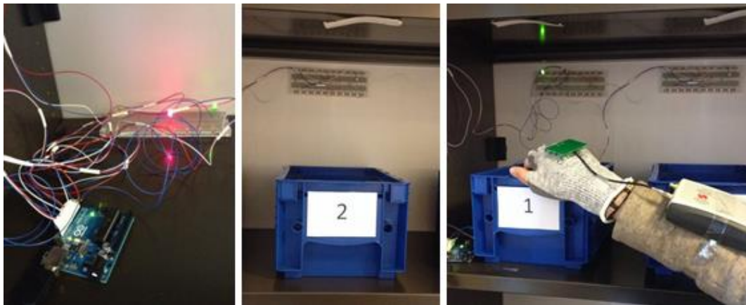
Figure 3.8. Details of the RFID pick-to-light system prototype (Left: Microcontroller and lights; Middle: stocking location with lights system and RFID tag; Right: operator wearing the RFID glove while entering a stocking location).
