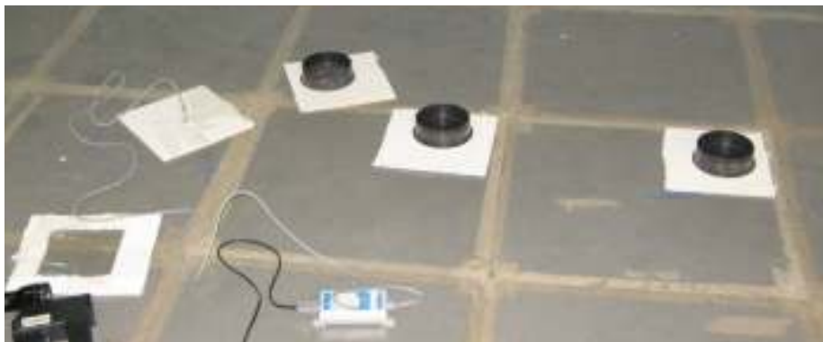
Figure 4-8 Air velocity measure with the omnidirectional anemometer
