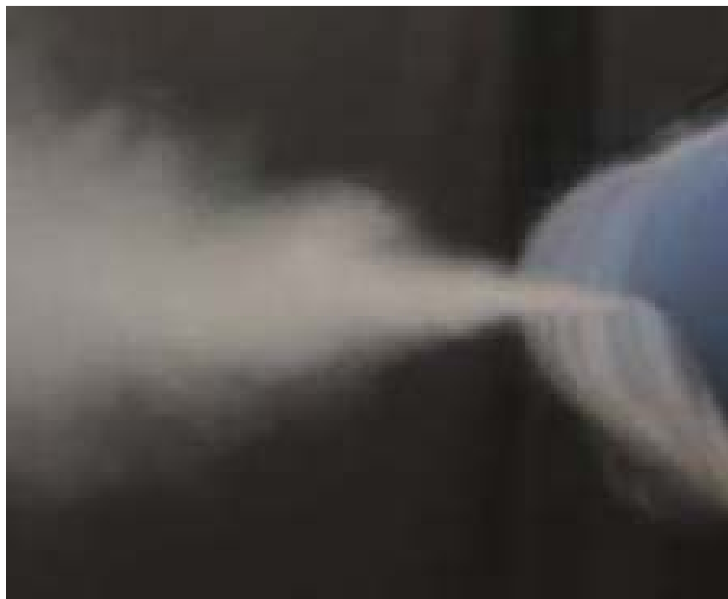
Figure 4-2 Smoke visualization of air leakage through the fabric (15).
