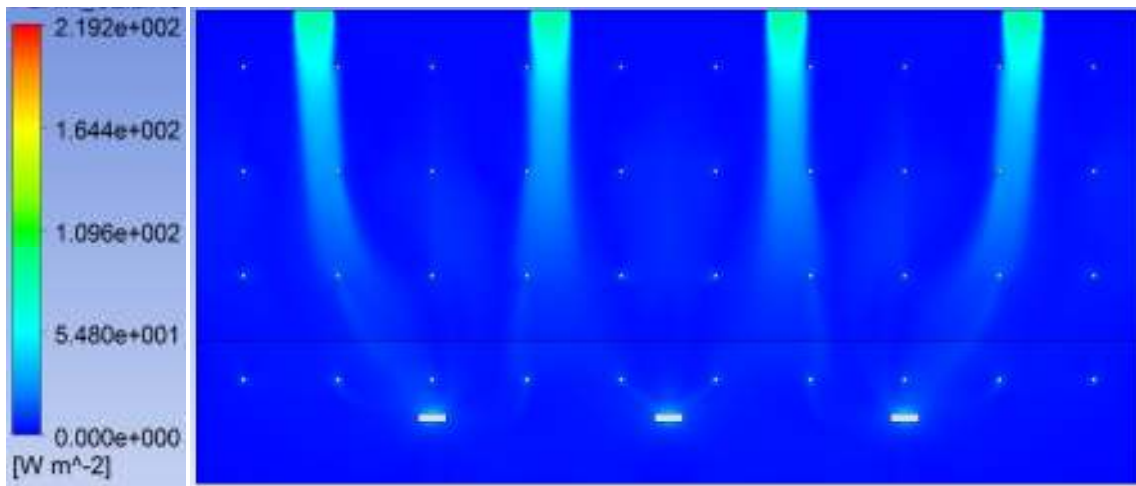
Figure 9-22 Configuration#1, 50% load conditions: ceiling heat flux.
