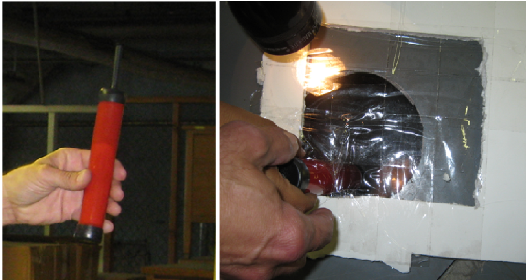
Figure 4-9 Air direction visualization with a smoke-stick
