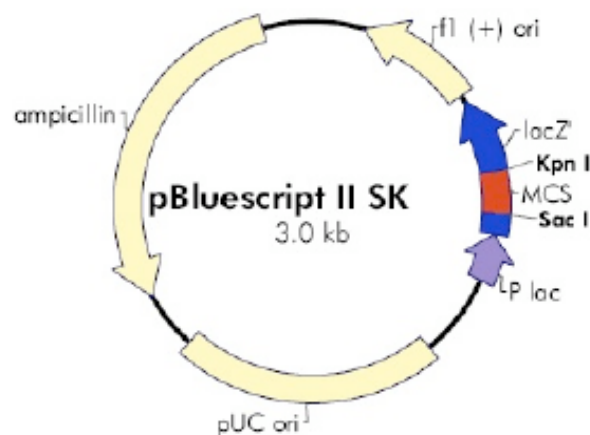
Fig.3.2: pBS plasmid 3,000 bp, MCS multiple cloning site 653-760 bp, http://image.hudsonalpha.org/html/libs/pBluescriptIISK+map.pdf
