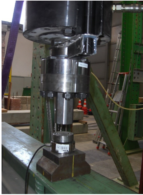
Figure 3.3: load cells utilized in the system. Upper cell with 30 ton capacity; lower cell with 10 ton capacity
