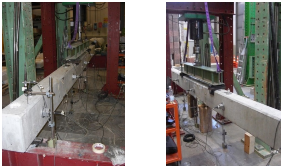
Figure 3.10: Load process of Beam 1
