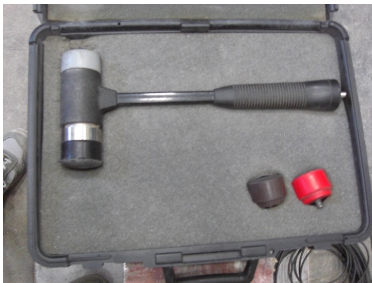
Figure 5.1 Impulse hammer used for dynamic tests
