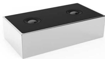
FIGURE 4.22: DUO MC stereo-camera used as the external reference camera to acquire images of the CUBE and the FFT during the floating phase.
