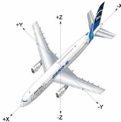
FIGURE 4.3: NED reference system of the Airbus A310 ZERO-G (©NoveSpace).
