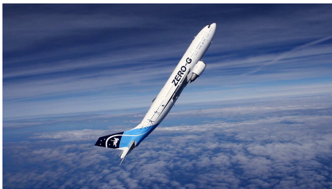
FIGURE 3.1: Parabolic flight manoeuvre. Different gravity levels are achieved during the manoeuvre. The low-gravity phase lasts about 22 s and it is reached at the peak of the parabola (©NoveSpace/CNES/DLR/ESA Id 324324).
