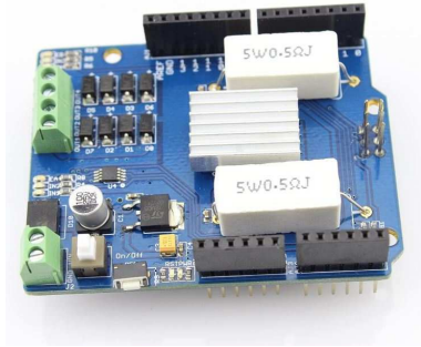
FIGURE A.5: Arduino UNO Motor Shield. This board has the same characteristics of the L298N in terms of output current and input voltage. In addition, it can monitor the current flowing in the coils.
