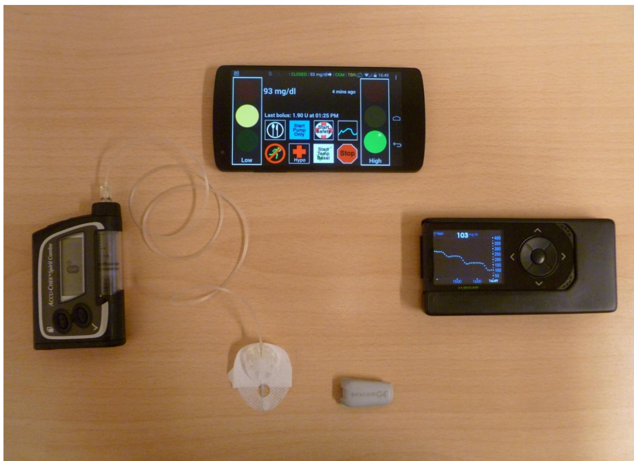
Fig 4: Our artificial pancreas model including DiAs, insulin pump (Accucheck Spirit Combo®, Roche Diabetes Care) and CGM (Dexcom G4®, Dexcom) inserted in relay box to allow Bluetooth communication between receiver and DiAs
