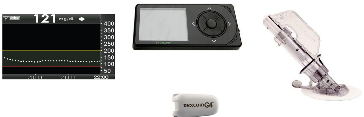
Fig 5: Dexcom G4 Continuous Glucose Monitoring system: on the right there is sensor with its applicator, on the left the transmitter and the receiver where patient could visualize glycemic values.
