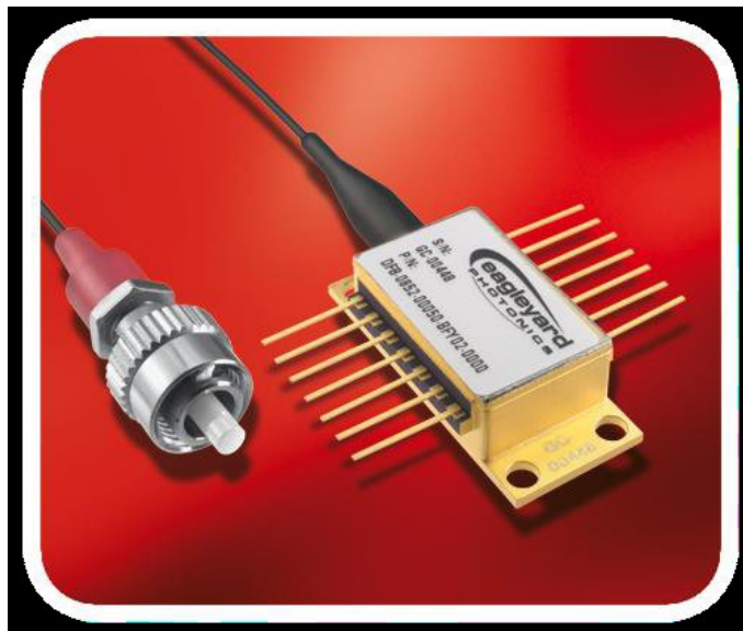
Figure 7.2: A fiber pigtailed DFB laser. The butterfly casing is very common in the telecommunications environment, usually provided with built in TEC element, temperature sensing thermistor and reference photodiode.
