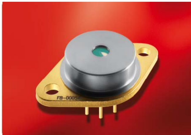
Figure 7.3: A high power (over 50mW) DFB laser. The heavy TO3 casing (originally developed for power transistors) provides all the features needed for thermal and power control, as well as a good thermal interface for heatsinks.
