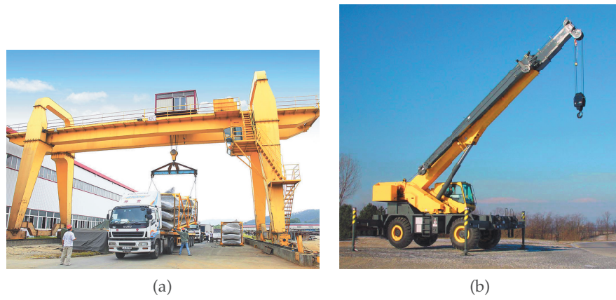
Figure 6: Gantry crane (a) and Mobile crane (b).
