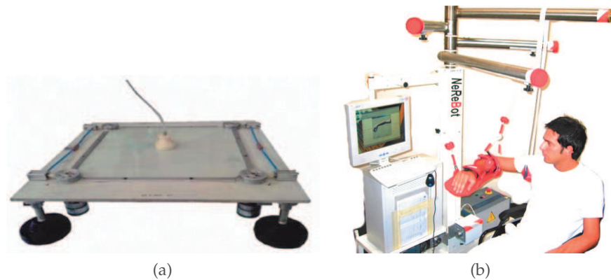
Figure 15: Prototype of cable robot developed at the University of Padua: Feriba (a) and Nerebot (b).
