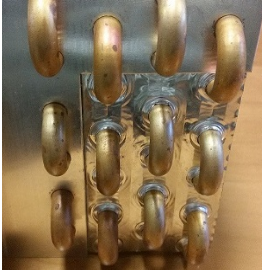
Fig. 4.11 Bare aluminium fin surface coating
