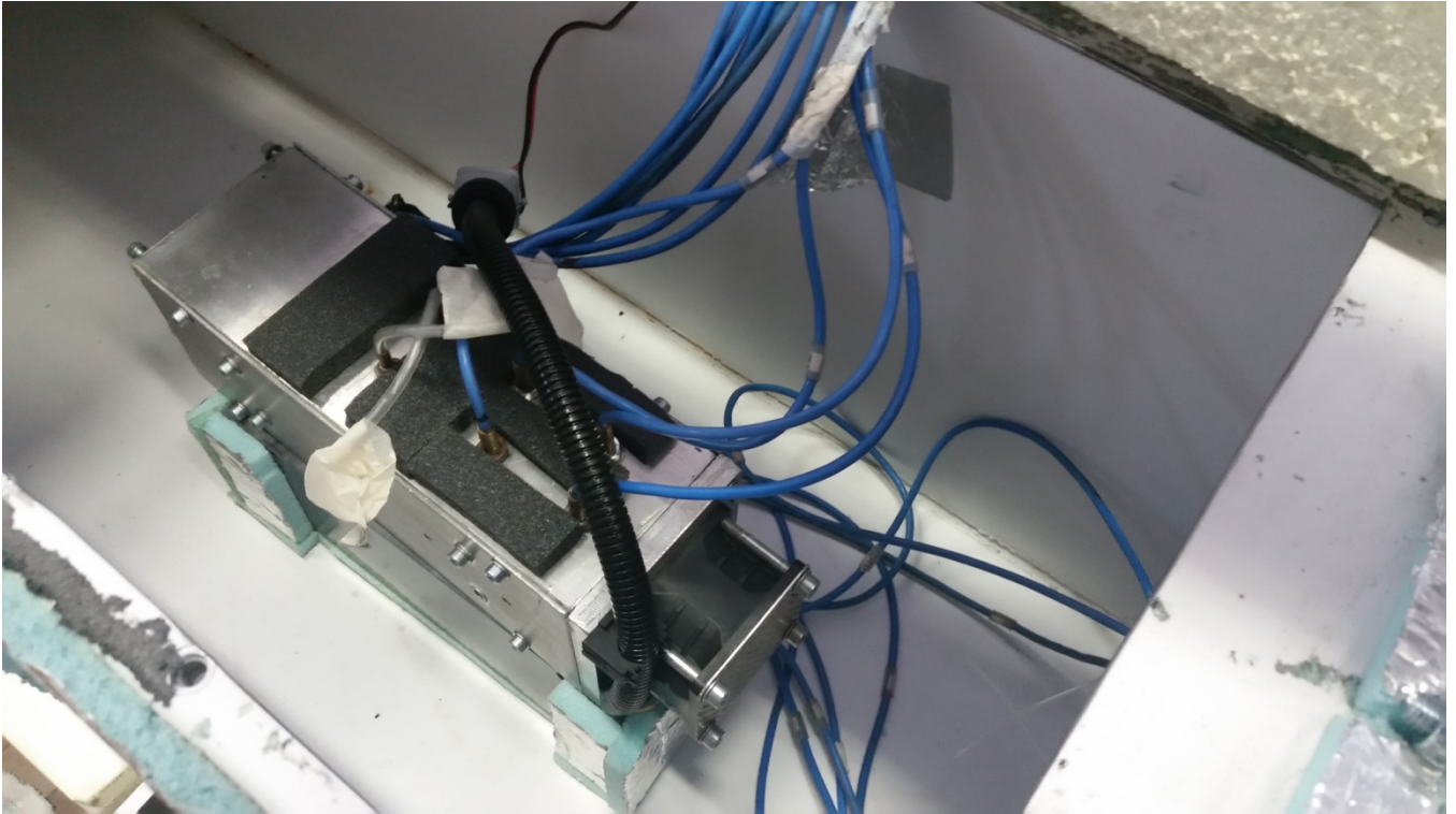
Fig. 5.25 Psychrometer final arrangement
