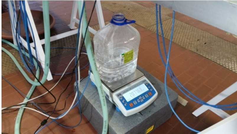
Fig. 5.27 Condensate measurement set up
