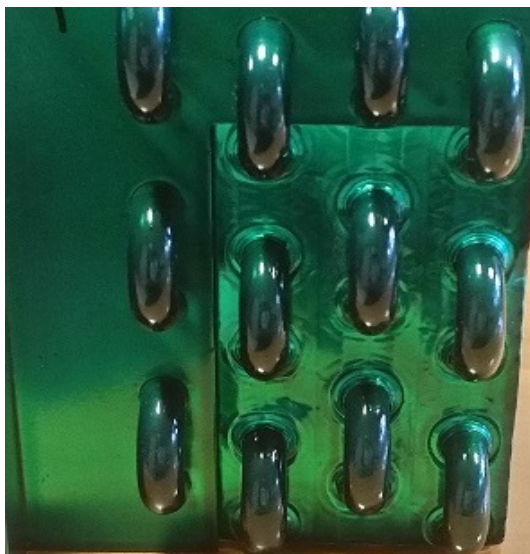
Fig. 4.13 Hydrophobic fin surface coating
