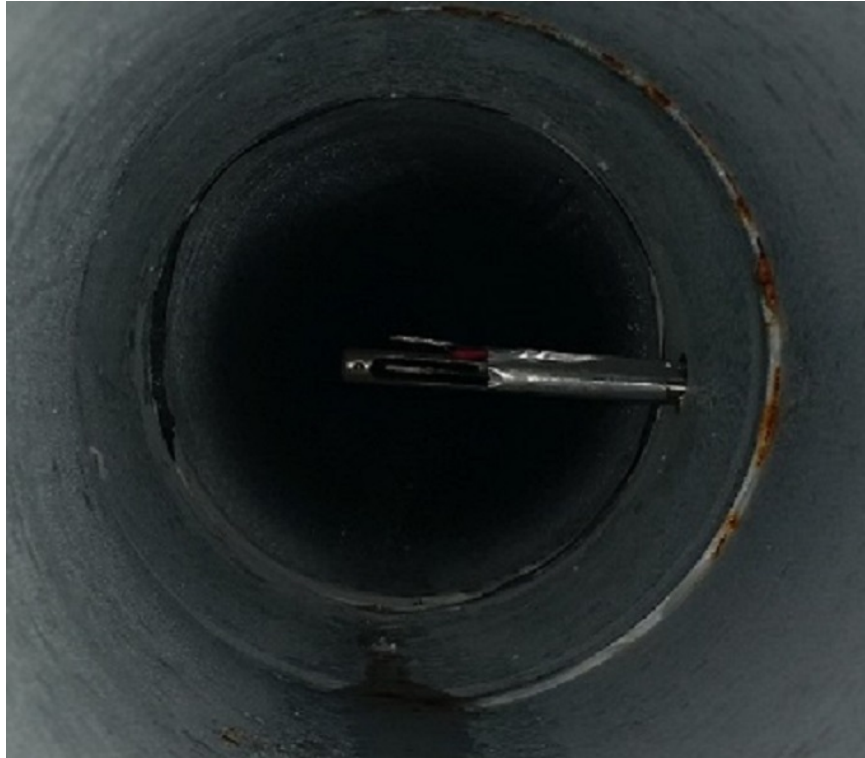
Fig. 5.25 Anemometer sensing element
