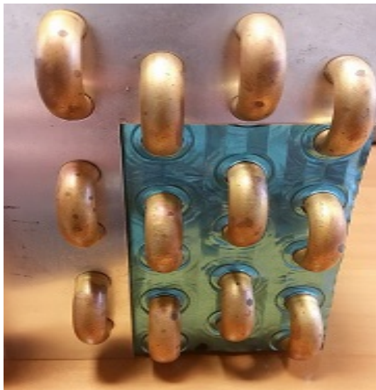
Fig. 4.12 Hydrophilic fin surface coating
