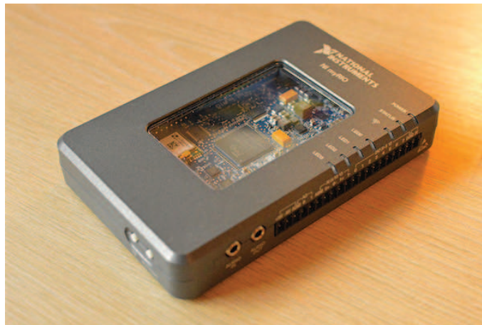
Figure 3.14: The configurable input-output myRIO-1900 device used to perform the closed loop control of the flow control valve.
