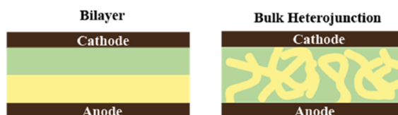
Figure 1.2 Schematic representation of the bilayer and BHJ architectures for polymer solar cells.
