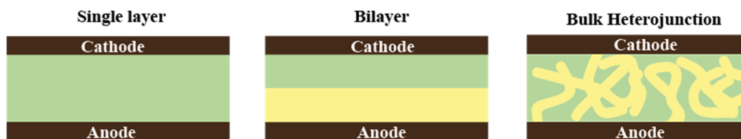
Figure 1.1 Schematic representation of single layer, bilayer and bulk heterojunction solar cells.
