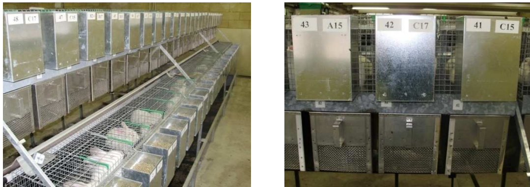
Figure 5. Experimental cages for in vivo digestibility trials and details of digestibility cages with removable feeders and baskets for the faeces collection.
