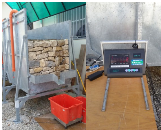
Figure 3.8. Outlet of the model where the water is collected and weighted by the scale
