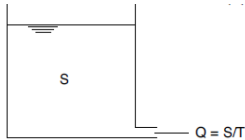
Figure 3.38. Conceptual schematization of a linear store.
