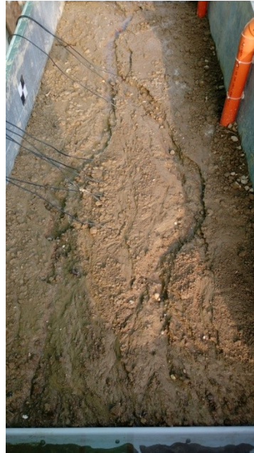
Figure 3.55. Erosions processes and channelization in small rills
