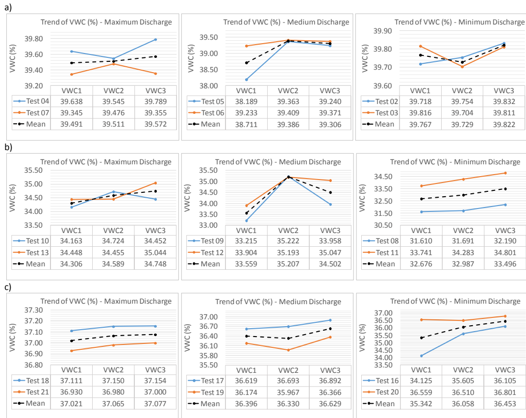
Figure 3.27. Overall Volumetric Water content for min, mean and max input discharges: a) 3% slope, b) 6% slope, c) 9% slope. The dashed black lines are obtained by averaging the results of each pairs of tests.
