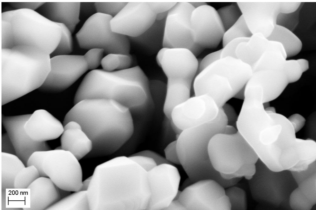
Figure 11, SEM image of XC72 impregnated with titanium isopropoxide, C:Ti ratio 1,75:1, treated at 1350°C for 3 hours
