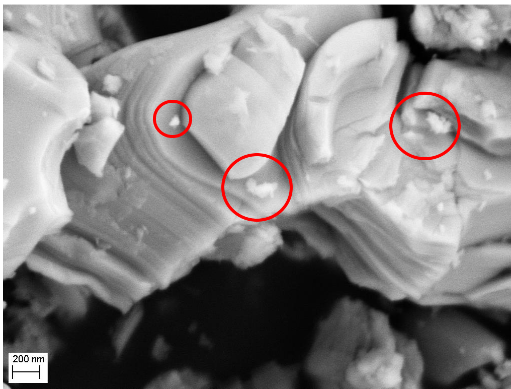
Figure 200, SEM image of the core part of TiC and Ti 2 AlC powders with molar ratio of 1:0.7, ball milled at 300 rpm for 18 hours and sintered at 1350°C for 2 hours with a vacuum stage, core from big volume
