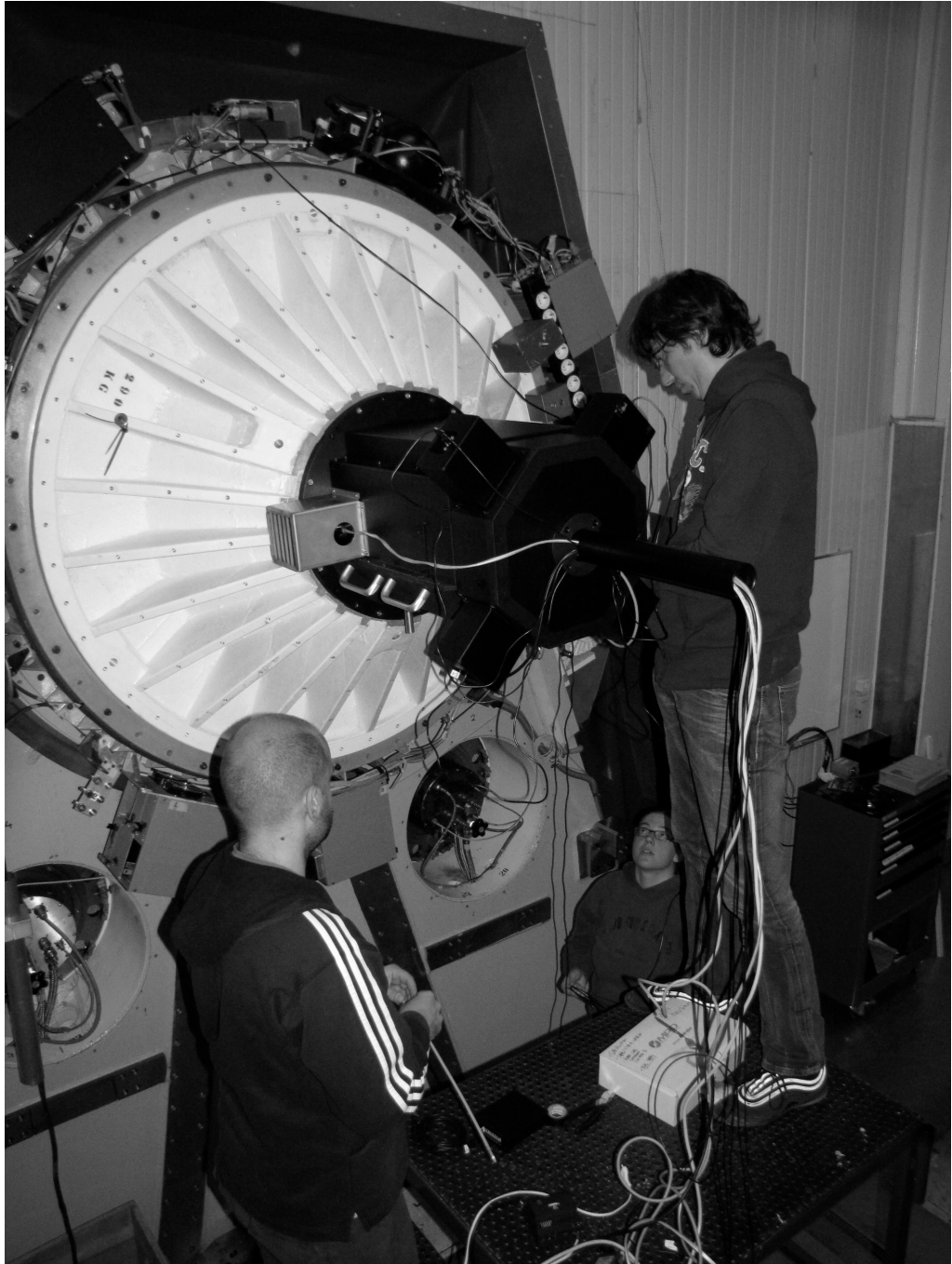
Figure 3.1: Iqueye being mounted at the NTT in La Silla (Credit: Naletto).
