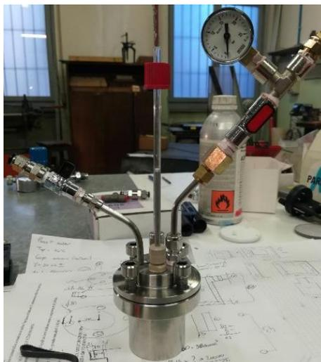
**Figure 8.6.** The SS304 reactor used for *e*ATRP of MA in the mechanical facility of the Department of Chemical Sciences.
