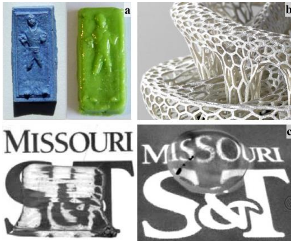
Fig. 3.1 - Attempts of AM with glass: powder-bed based approaches by (a) Klein, S. et al. and (b) ExOne; (c) wire fed SLM [5,6,10].
