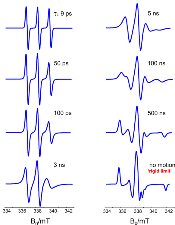
Figure 2.12: Changes in the lineshape of a room temperature CW-EPR spectrum with the correlation time. Spectra are simulated using Matlab EasySpin “chili” using static parameters \mathbf{g}=[2.008, 2.006, 2.003] and \mathbf{A}=[20, 20, 85] MHz.
