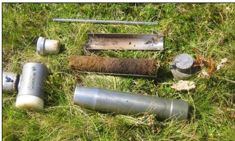
**Figure I.5.** Core samples collector for analyzing root characteristics.
