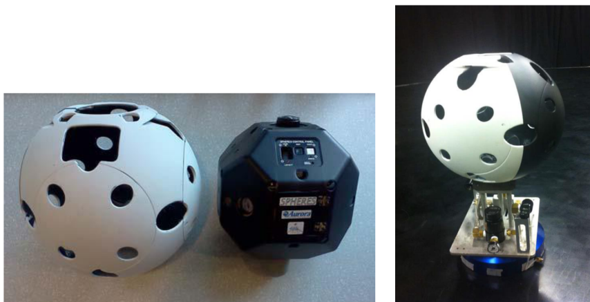
Figure 7.3: OS Shell with a SPHERE satellite for comparison (left); OS on an air bearing support structure (right) (courtesy of [82]).
