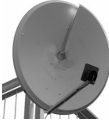
Figure 8.3: Twisted parabolic antenna for generating \ell = 1 OAM channel.
