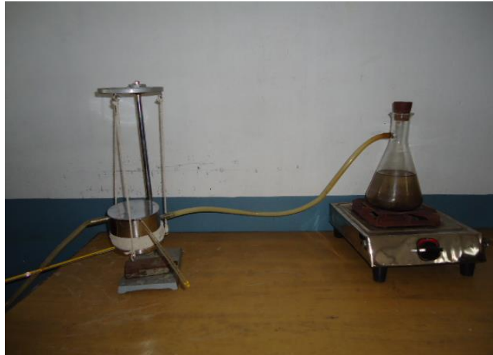
Fig. 6. 4: Setup of sampling tile in Lee's method
