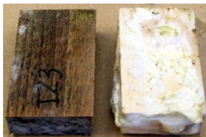
Fig. 5. Biological attack of C. Puteana on tannin-boron treated (left) and untreated (right) Beech specimens
