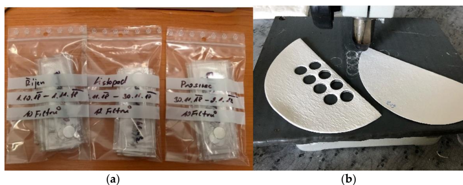
Figure 4. (a) A packed set of exposed filter samples, and (b) the preparation of samples using the special automatic punching head.
