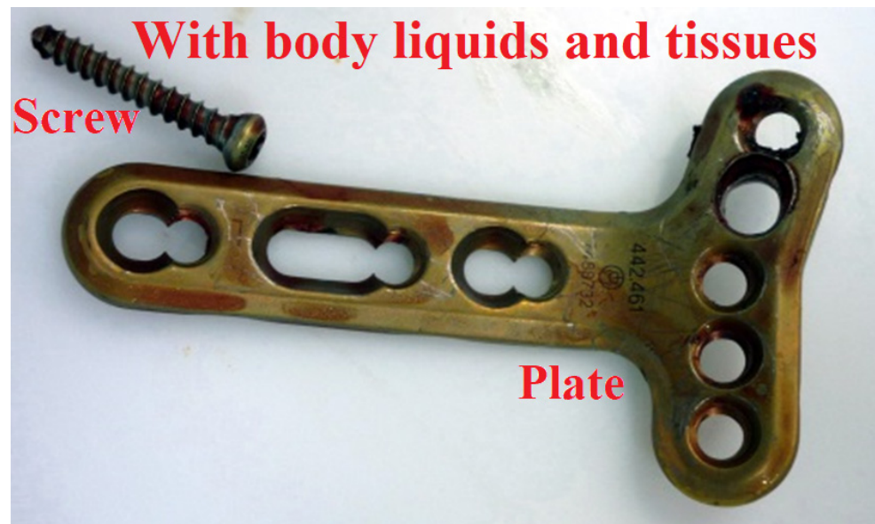
Figure 15. Angularly stable plate with locking bone screws removed from the human wrist.
