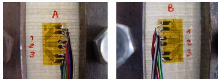
Fig. 9 – Particular of the strain gauges installed on the specimen surface on two different sides of the specimen
