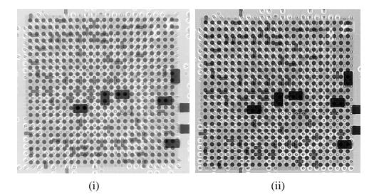
Figure 22. (i) Post Soak (ii) Post Bake X-Ray Image Top View
