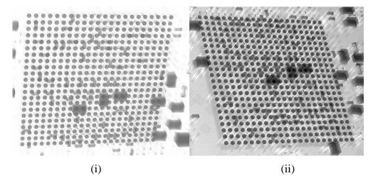
Figure 48. P5 Area 1 (i) Post Soak (ii) Post Bake X-Ray Image Angle View
