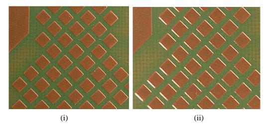
Figure 42. (i) Post Soak (ii) Post Bake Visual Image of Surface Area 2 of P4.
