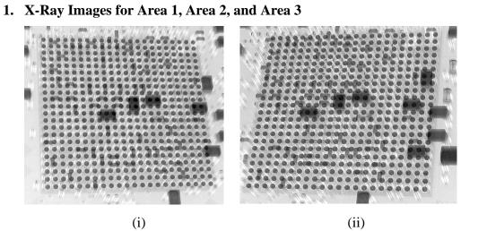
Figure 43. P2 Area 1 (i) Post Soak (ii) Post Bake X-Ray Image Angle View.
