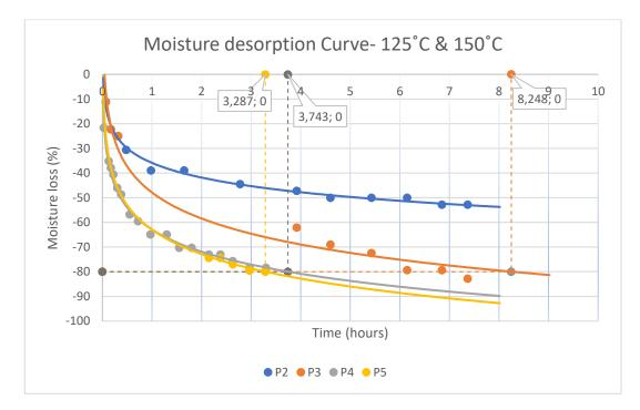
Figure 17. Moisture Desorption Curve of P2-P5.
