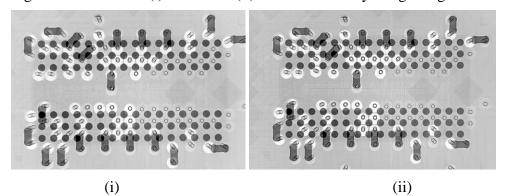
Figure 50. P3 Area 2 (i) Post Soak (ii) Post Bake X-Ray Image Top View
