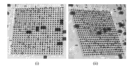
Figure 46. P4 Area 1 (i) Post Soak (ii) Post Bake X-Ray Image Angle View
