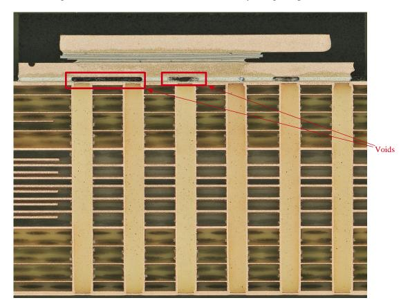
Figure 37. Cross-section overview at 140X magnification of Area 3.
