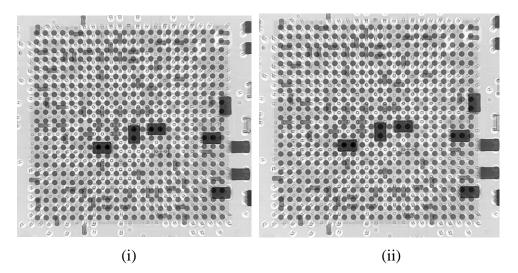
Figure 44. P3 Area 1 (i) Post Soak (ii) Post Bake X-Ray Image Top View.
