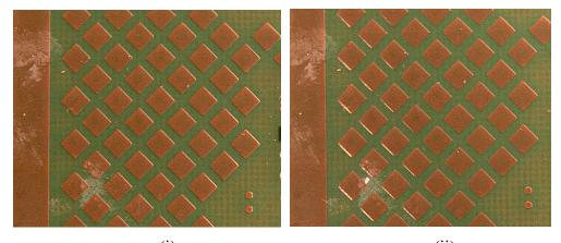
(i) (ii) Figure 63. (i) Post Soak (ii) Post Bake Visual Image of Surface Area 2 of P3
