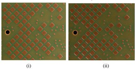
Figure 40. (i) Post Soak (ii) Post Bake Visual Image of Surface Area 1 of P4.
