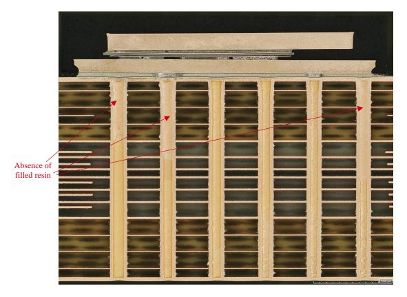
Figure 34. Cross-section overview at 140X magnification of Area 3.
