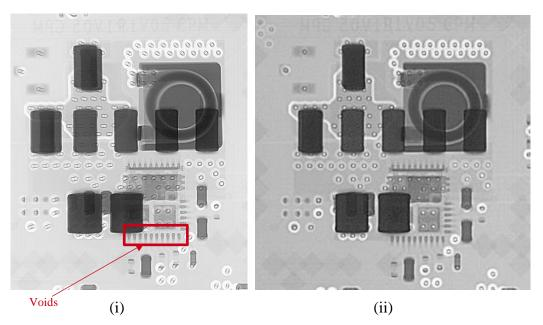
Figure 36. (i) Post Soak (ii) Post Bake X-Ray Image Top View
