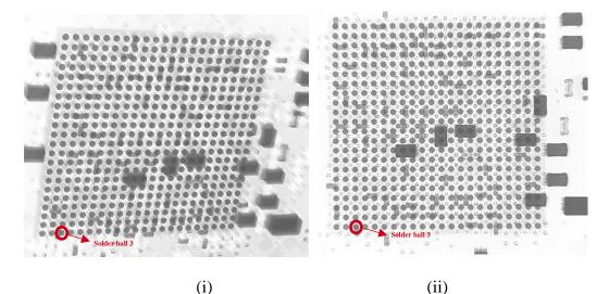
Figure 18. Pre-Soak X-Ray Reference Image (i) Top View (ii) Oblique View.
