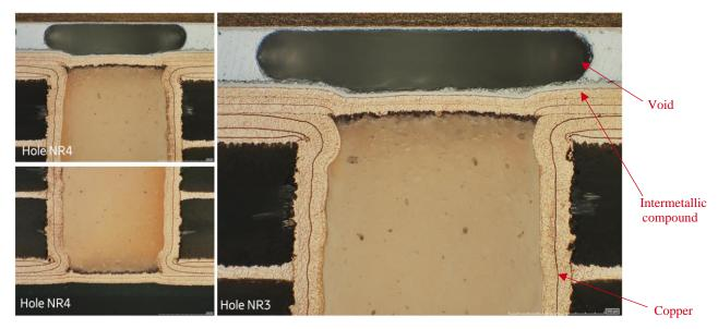
Figure 32. Hole numbers 3 and 4 in cross-section of Area 3.
