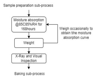
Figure 11. Sample pre-conditioning sub-process.
