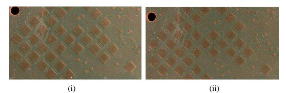
Figure 62. (i) Post Soak (ii) Post Bake Visual Image of Surface Area 1 of P5
