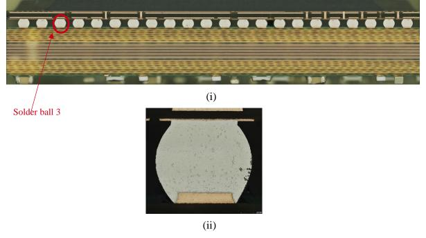
Figure 21. (i) Cross-section overview at 140X magnification of Area 1 (ii) Overview of solder ball 3 showing no signs of defect.
