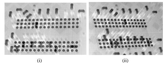
Figure 52. P4 Area 2 (i) Post Soak (ii) Post Bake X-Ray Image Angle View
