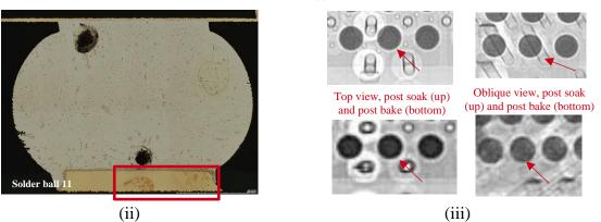
Figure 23. (i) Cross-section overview at 140X magnification of Area 1 (ii) Overview of solder ball 11 (iii) Solder ball 11 in post-soak and post-bake X-Ray Image.
