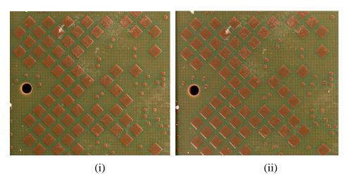
Figure 61. (i) Post Soak (ii) Post Bake Visual Image of Surface Area 1 of P3
