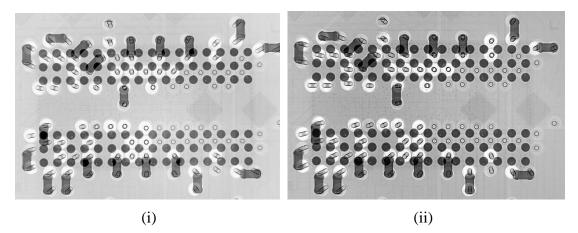
Figure 28. (i) Post Soak (ii) Post Bake X-Ray Image Top View
