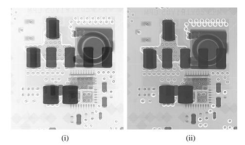
Figure 56. P3 Area 3 (i) Post Soak (ii) Post Bake X-Ray Image Top View
