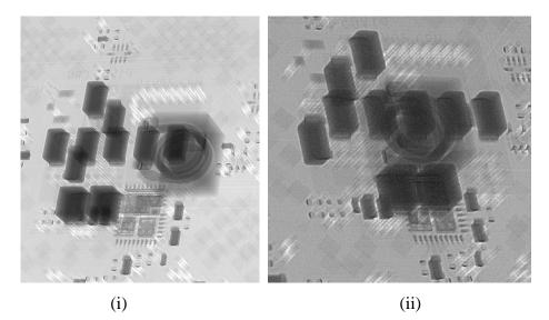
Figure 58. P4 Area 3 (i) Post Soak (ii) Post Bake X-Ray Image Angle View
