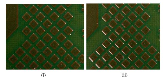
Figure 41. (i) Post Soak (ii) Post Bake Visual Image of Surface Area 2 of P2.
