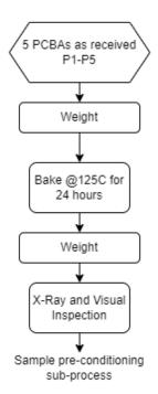
Figure 10. Sample preparation sub-process.
