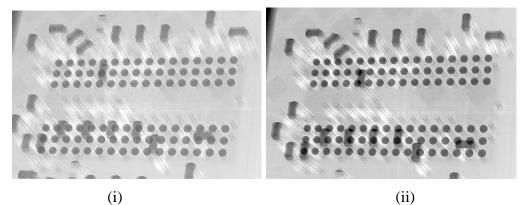
Figure 51. P3 Area 2 (i) Post Soak (ii) Post Bake X-Ray Image Angle View
