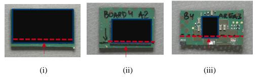
Figure 14. Cross-section areas for (i) Area 1 (ii) Area 2 (iii) Area 3.
