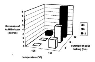
Figure 2. Impact of baking on the IMC thickness.
