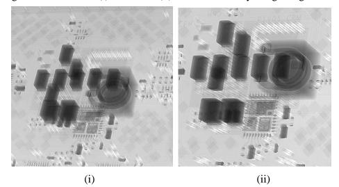
Figure 55. P2 Area 3 (i) Post Soak (ii) Post Bake X-Ray Image Angle View
