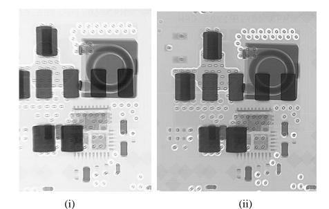
Figure 59. P5 Area 3 (i) Post Soak (ii) Post Bake X-Ray Image Top View
