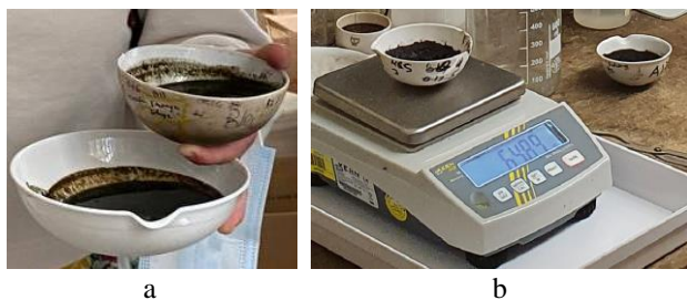
Figure 8 – Image of the digestate appearance obtained after anaerobic digestion of plant substrate and phosphogypsum: a – rare phase; b – solid phase
