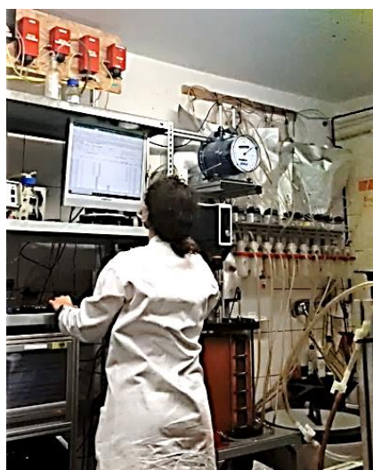
Figure 3 – Lab stand for anaerobic digestion
