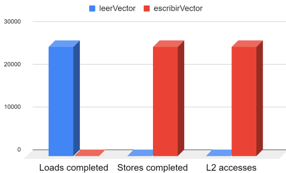
Figura 7: Accessos a L2 pel Write-Through
