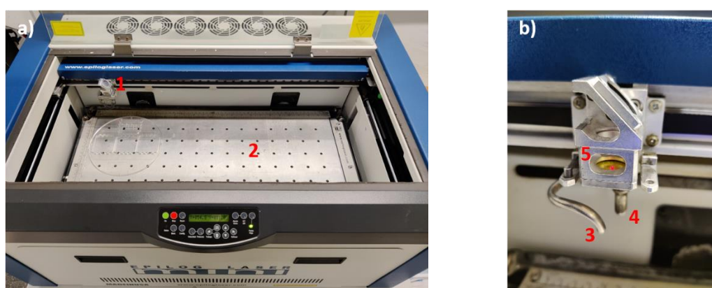
Figure 10. a) Epilog Legend Mini 24 (1: Lens moving head. 2: Sample stage.). b) Lens moving head (3: Air Assist expeller. 4: Autofocus sensor. 5: Focusing lens).
