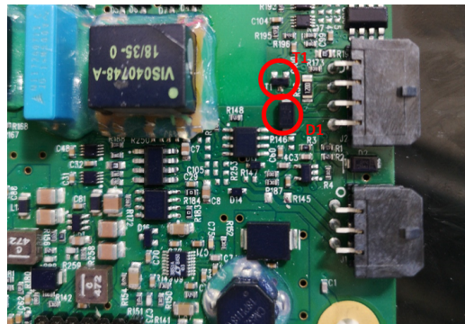
Figure 45: Boot Out transistor and TVS diode on BMU PCB
