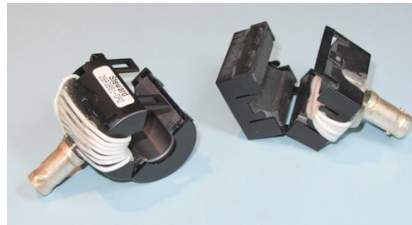
Figure 32: Examples of DIY probes based on clamp-on ferrite chokes.
