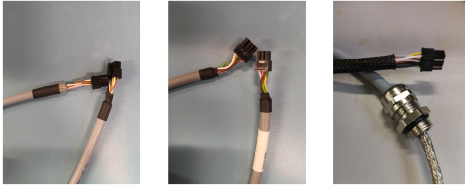
Figure 54: Cables used for RS-485 communication interface
