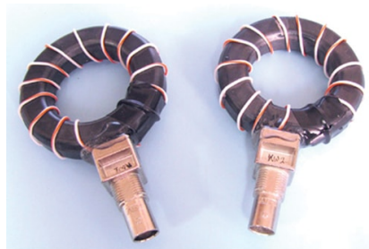
Figure 33: Examples of DIY probes based on a large toroid core
