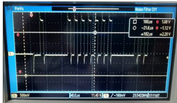
Figure 61: Offset RS-485 differential signal
