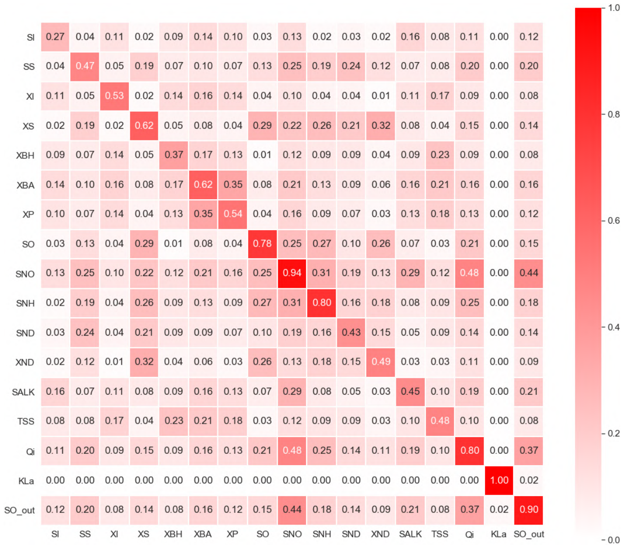
Figure 3.6: Mutual information matrix of the data from the entrance to the fifth tank, its oxygen transfer coefficient ( K_{La5} ), and the dissolved oxygen at the exit of said fifth tank ( S_{O,5} ).
